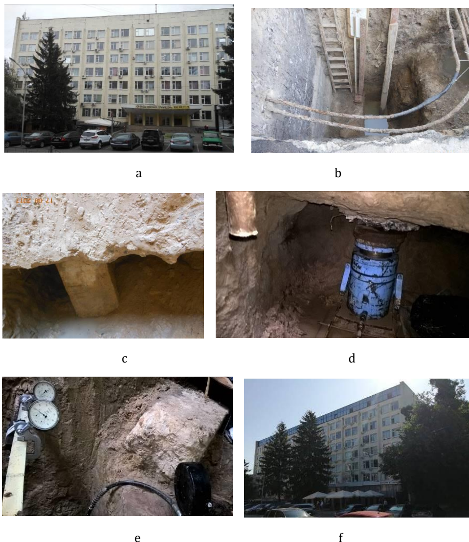
Figure 4. Engineering and geological investigations of an eight-storey building with pile foundations: a - building before superstructure; b - borehole from which the building foundations were examined and static load tests of a single pile that had been loaded for a long time were performed in pile group; c - view from the borehole of the pile in pile group; d - static load tests of a single pile in pile group (hydraulic jack between the pile head and the bottom of the pile cap); e - static load tests of a single pile in pile group (reference system and deflectometers for fixing the pile settlements during its static tests); f - building after its superstructure by one floor.
