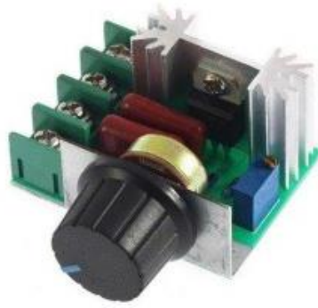
Figure 2.7 – Dimmer with manual adjustment
