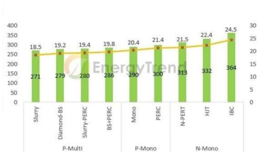
Figure 1.6 - Graph of efficiency of solar cells and power of panels depending on the technology used
