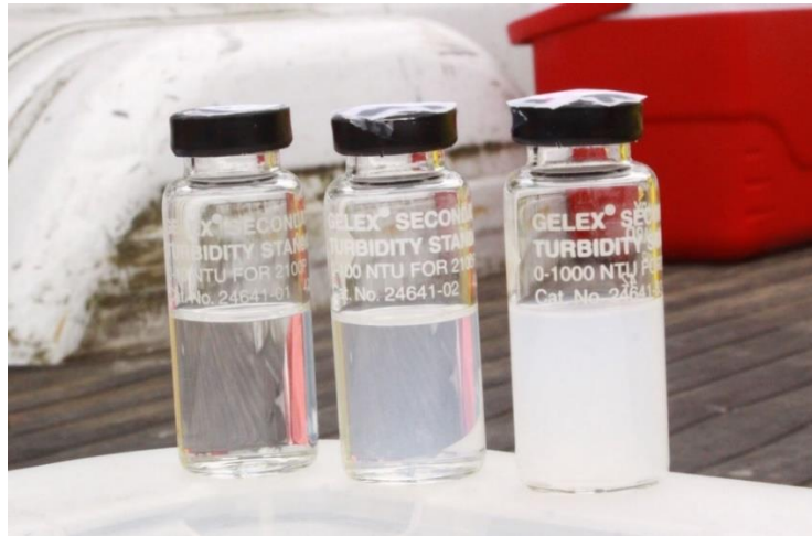
Figure 3.19 – Image for visual approximation of NTU pollution value
