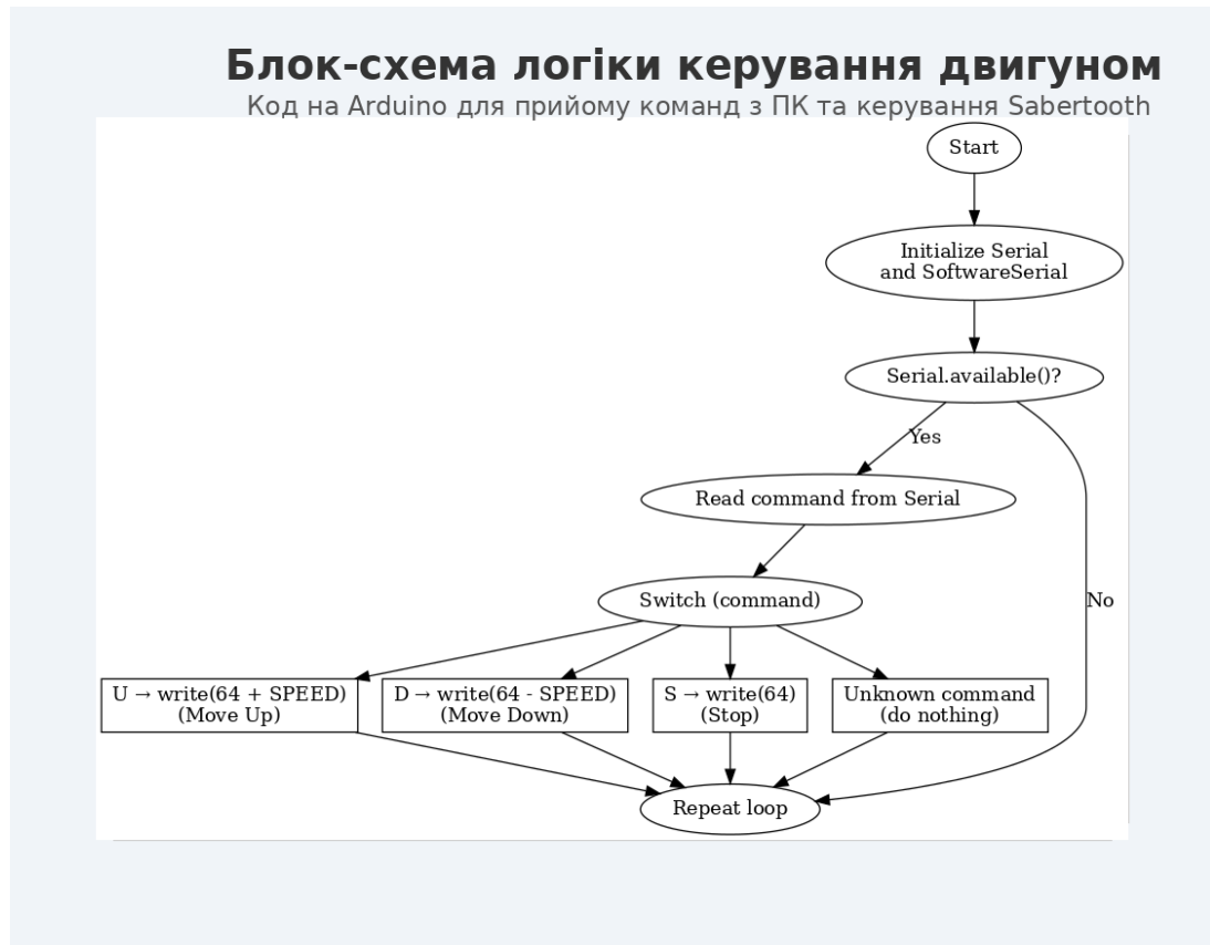
Figure 3.6 – Flowchart drive control
