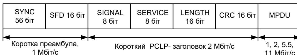
Picture 1.8 Short header of 802.11.b network frames
