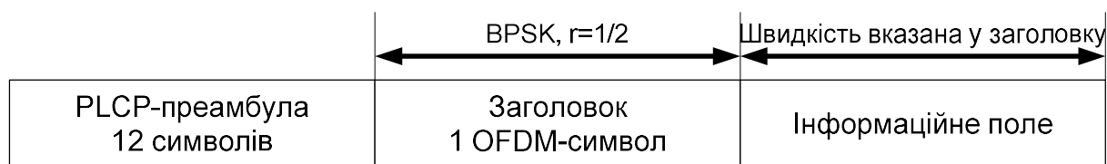
Picture 1.2 Structure of the physical layer header of the IEEE 802.11.a standard
