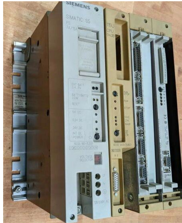
Figure 1.3 – Siemens S5-115U Controller
