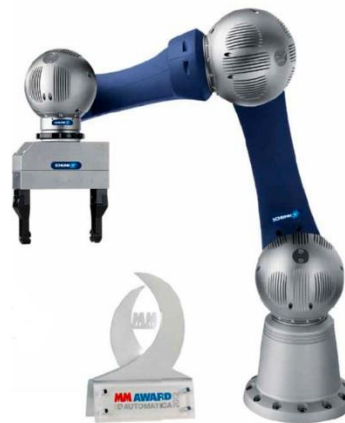
Figure 1.13 - Six-stage robot LWA 4.6 SHUNK
