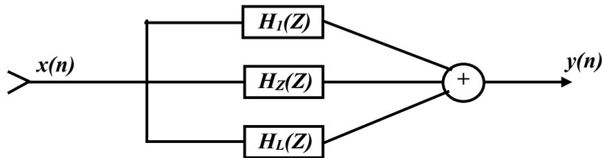
Fig. 2.67. Structural diagram of parallel implementation of DF
