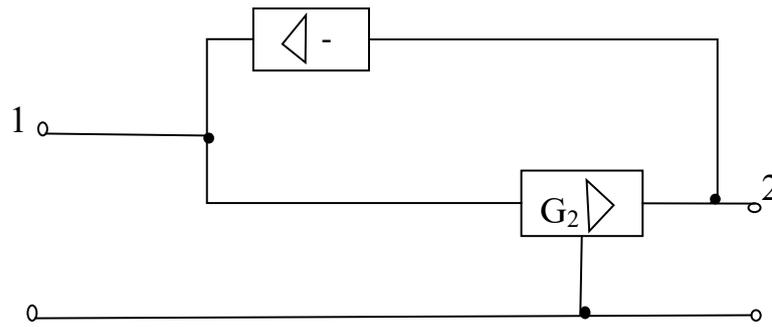
Fig. 2.49. Functional scheme of the gyrator
