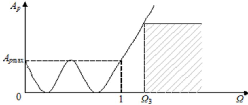
Fig. 2.10. The working attenuation graph of the Chebyshev filter
