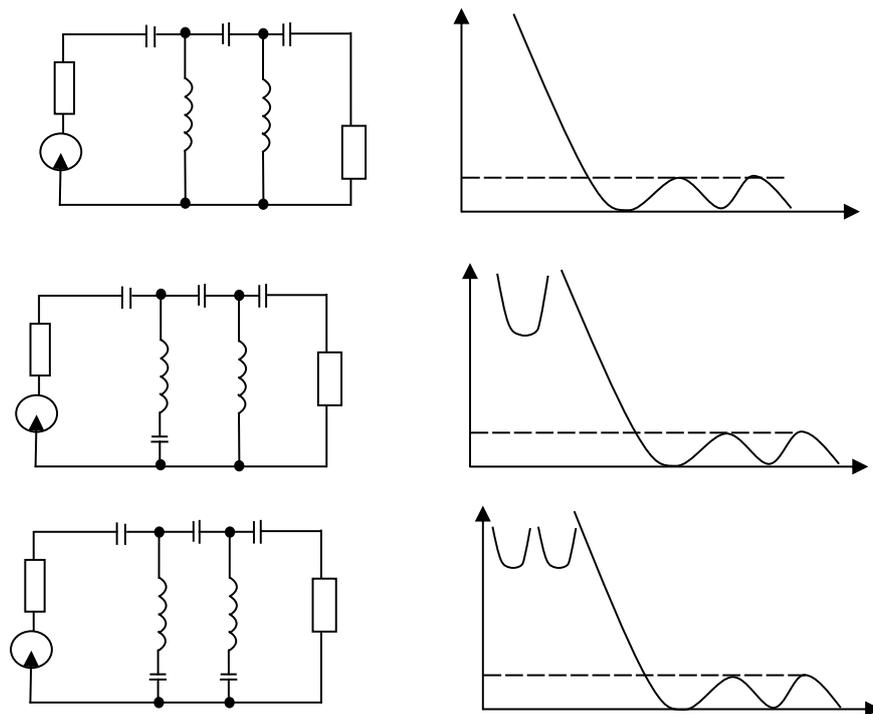
Fig. 2.21. Attenuation characteristics of high-pass filters with equal-wave attenuation characteristics
