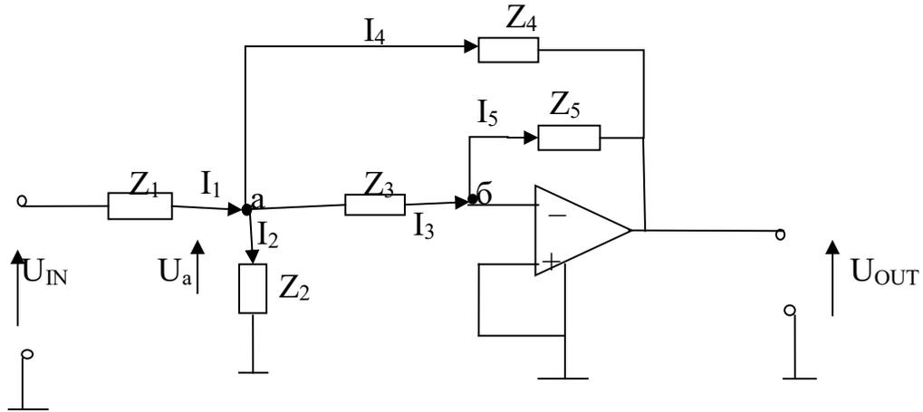
Fig. 2.44. Implementation of the 2nd-order link of the low-pass filter in the form of an active RC-filter on the operational amplifier
