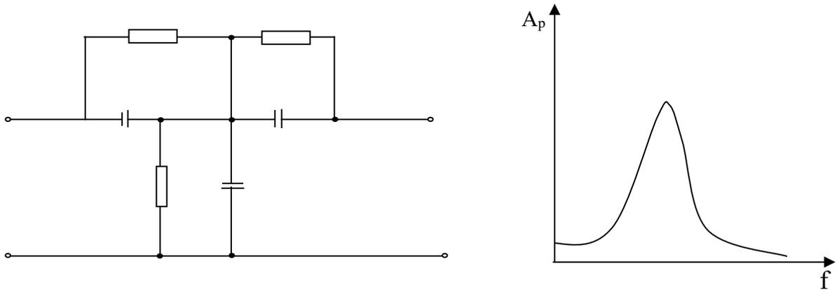
Fig. 2.41. Attenuation characteristic of the rejection filter
