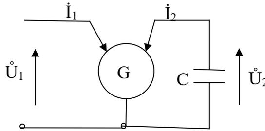
Fig. 2.48. Turning on the gyrator to simulate inductance
