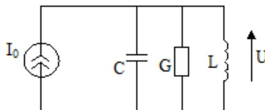
Fig. 1.3. An inductor and a capacitor are connected in parallel
