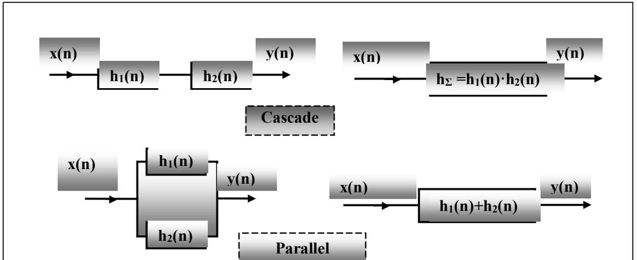
Fig. 2.57. Cascading and parallel inclusion of discrete processing systems
