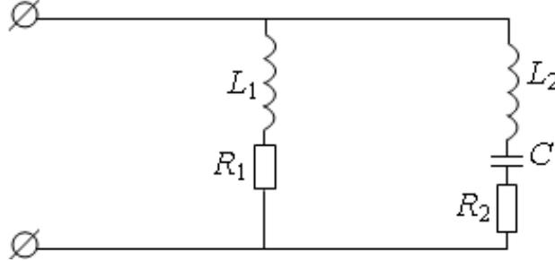
Fig. 1.24. Oscillatory circuit of the II type
