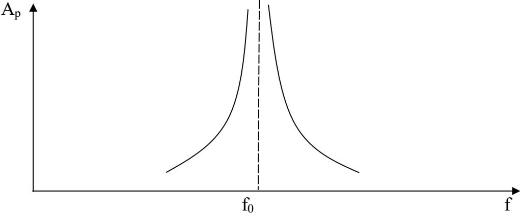
Fig. 2.24. Attenuation characteristics of the bandpass filter
