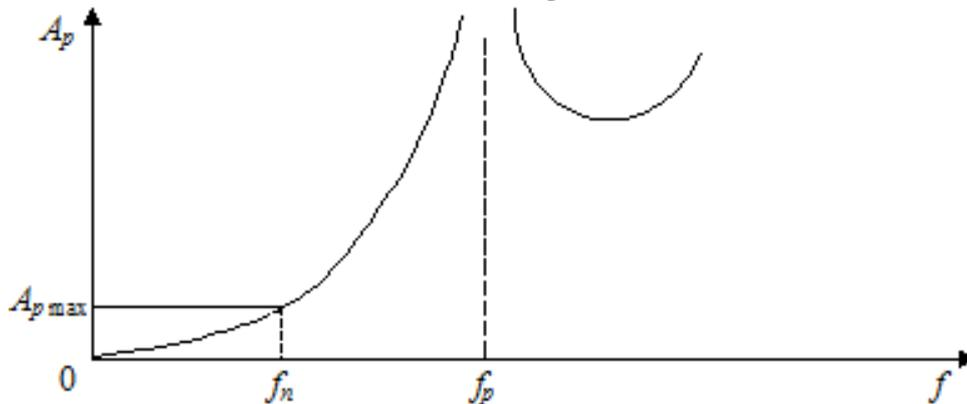
Fig. 2.15. Attenuation characteristics of filters with bursts
