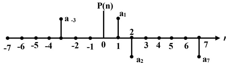
Fig. 2.55. Representation of a discrete sequence
