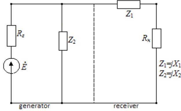
Fig. 2.5. The simplest L-shaped quadrupole
