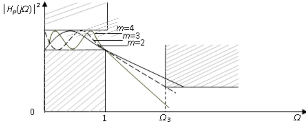
Fig. 2.11. AFC of the Chebyshev filter of different orders
