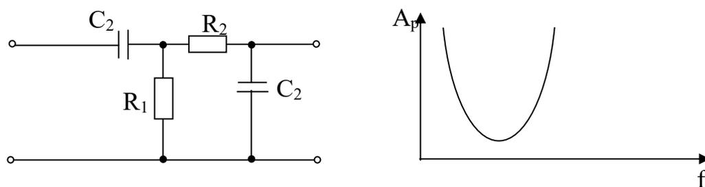
*Fig. 2.40. Attenuation characteristics of the bandpass filter*
