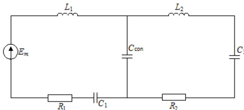
Fig. 1.17. Connected oscillating circuits with internal capacitive of the connection
