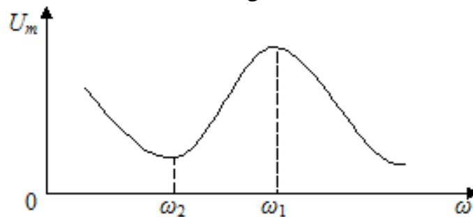
Fig. 1.27. AFC of the oscillating circuit of type III
