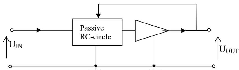
Fig. 2.42. Structural scheme of an active RC filter
