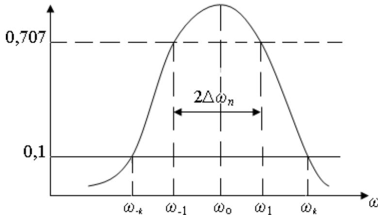
Fig. 1.15. AFC of the oscillating circuit
