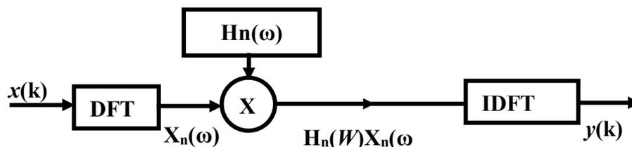
Fig. 2.68. The structural scheme of the parallel implementation of the DF
