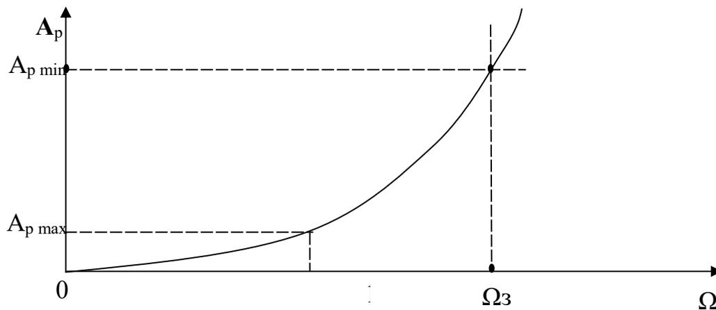
Fig. 2.28. Filter attenuation characteristic
