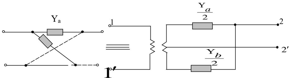
Fig. 2.33. Scheme of a bridge quadrupole
