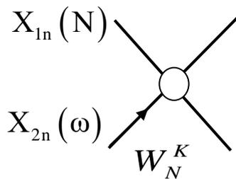
Fig. 2.69. Schematic representation of the operation “butterfly”
