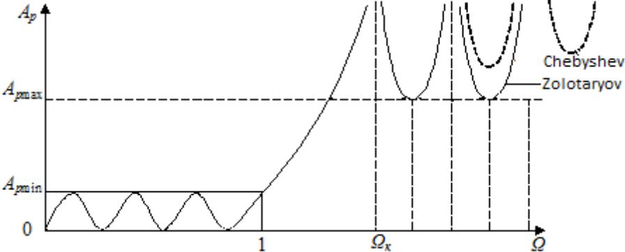
Fig. 2.17. Frequency dependence of filter attenuation with Zolotaryov characteristics
