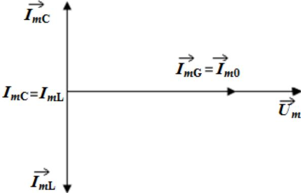
Fig. 1.5. Vector diagram of currents in a parallel oscillating circuit
