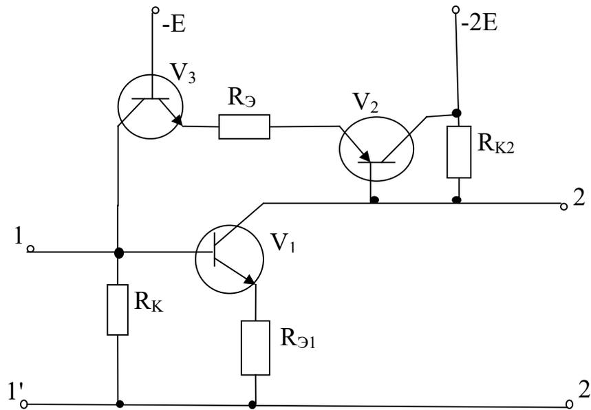
Fig. 2.50. Schematic scheme of the gyrator
