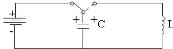
Fig. 1.2. Processes in a parallel oscillating circuit
