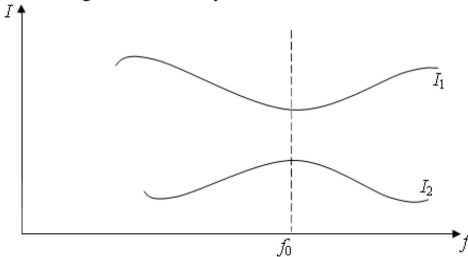
Fig. 1.23. Setting up linked circuits by changing the parameters of only the secondary circuit
