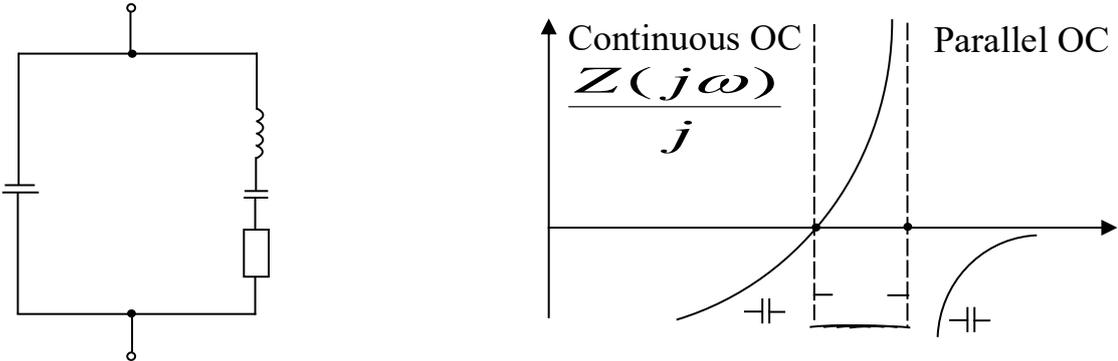
Fig. 2.31. Resonator replacement scheme
