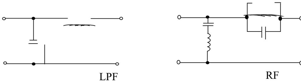
Fig. 2.25. Transition to the rejection filter
