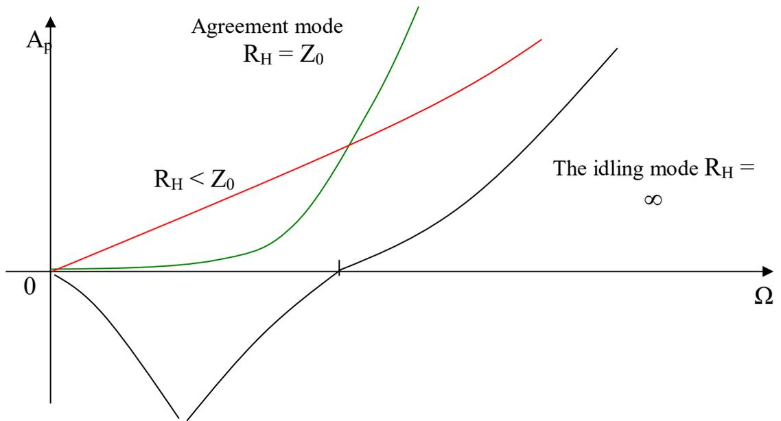
Fig. 2.30. Dependence of low-pass filter attenuation on load resistance
