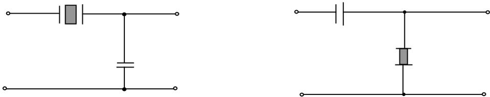
Fig. 2.32. The simplest filter links
