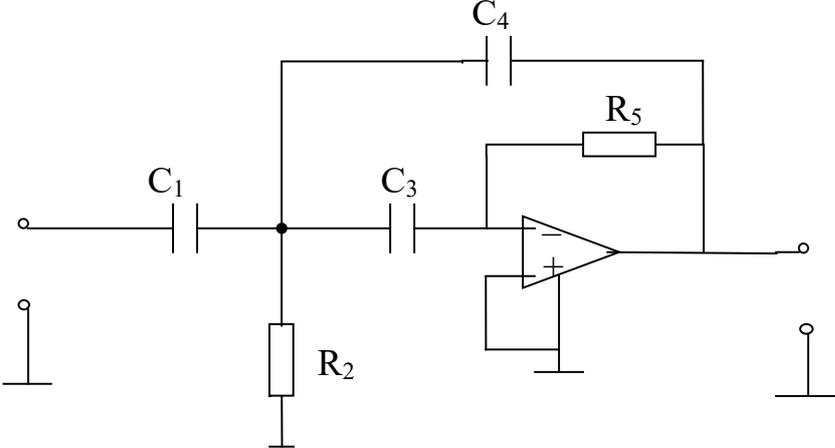
*Fig. 2.46. Scheme of a high-frequency RC filter of the 2nd order*
