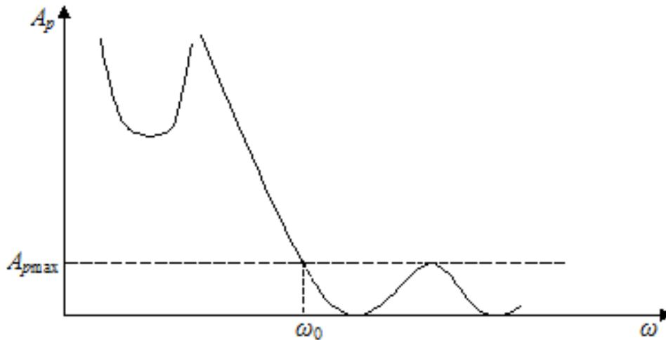
Fig. 2.20. Characteristics of attenuation of the high-pass filter
