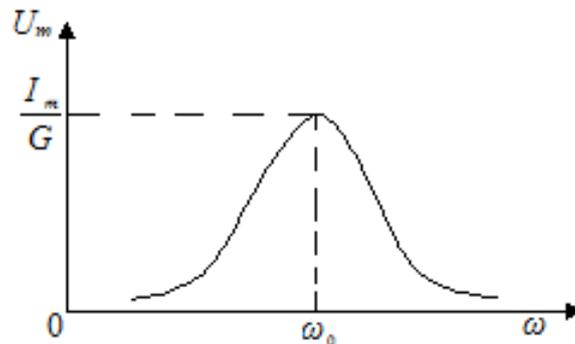
Fig. 1.9. Dependence of the voltage on the parallel oscillating circuit on the frequency
