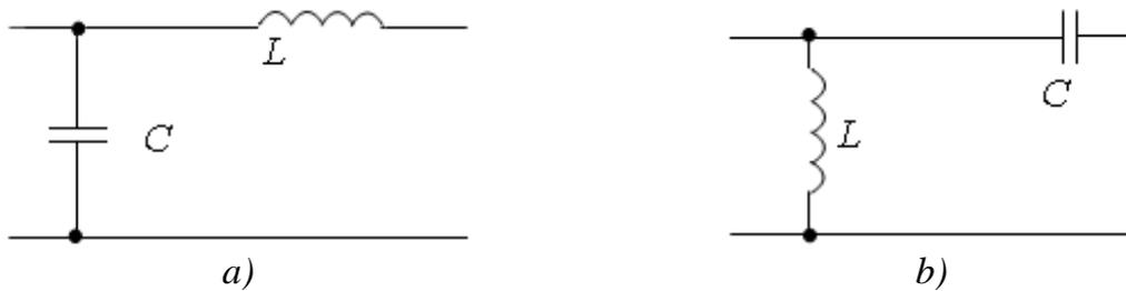
*Fig. 2.6. Links of electric filters*
