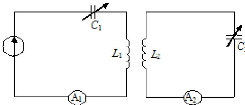
Fig. 1.21. Setting up connected circuits by changing the parameters of only the primary circuit
