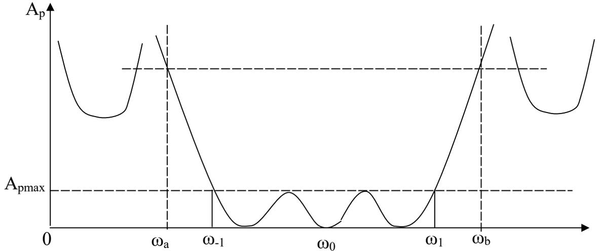
Fig. 2.23. Characteristics of BF attenuation
