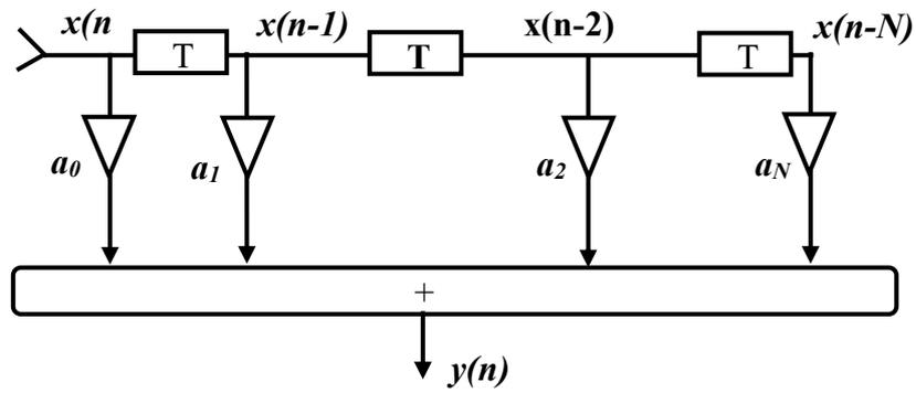
Fig. 2.62. Structural scheme of the FIR filter
