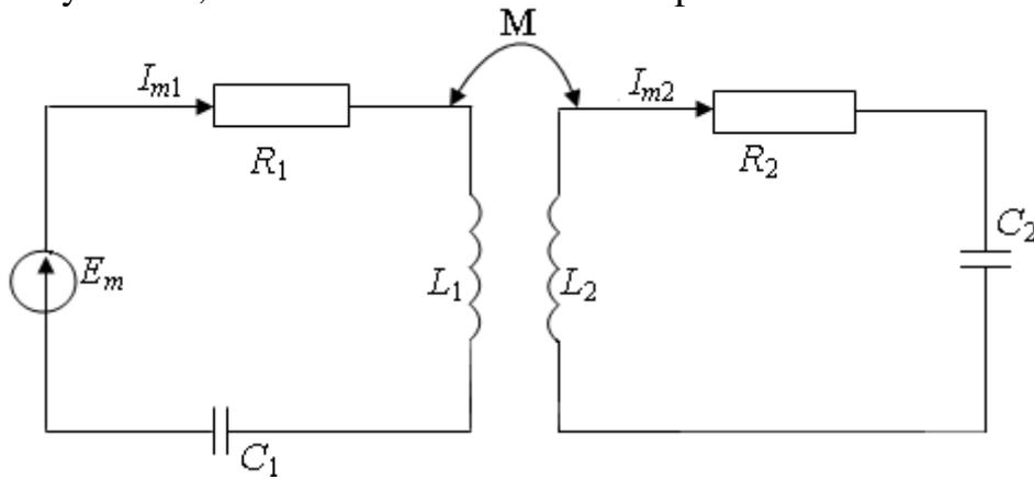
Fig. 1.18. Connected oscillating circuits with a transformer connection
