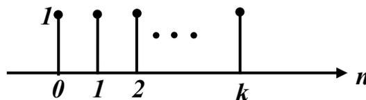
Fig. 2.54. A graphical representation of a discrete unit step sequence
