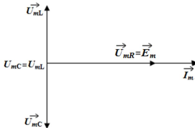
Fig. 1.7. The vector diagram of voltages in a series oscillating circuit
