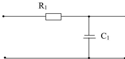
*Fig. 2.37. RC-filter of lower frequencies*
