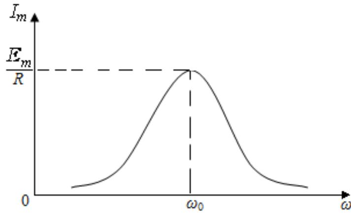
*Fig. 1.11. Dependence of the current amplitude through a series oscillating circuit on the frequency*
