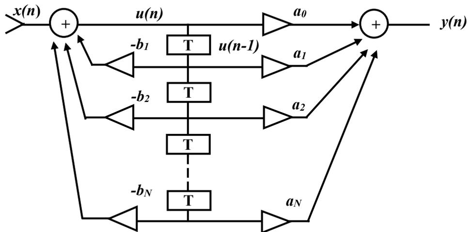
Fig. 2.65. Canonical structural scheme of the IIR filter
