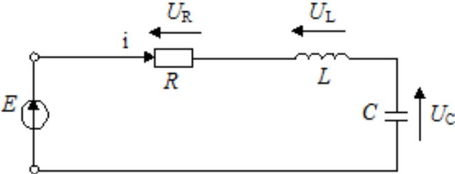
Fig. 1.6. A series oscillating circuit under the action of a HEF source
