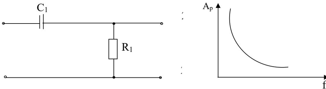
*Fig. 2.39. Characteristics of attenuation of the RC-filter of upper frequencies*
