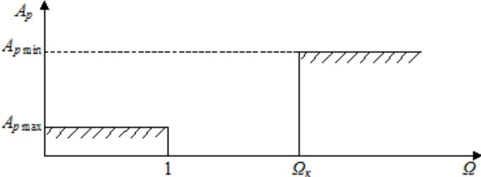
Fig. 2.16. LPF attenuation characteristics requirements
