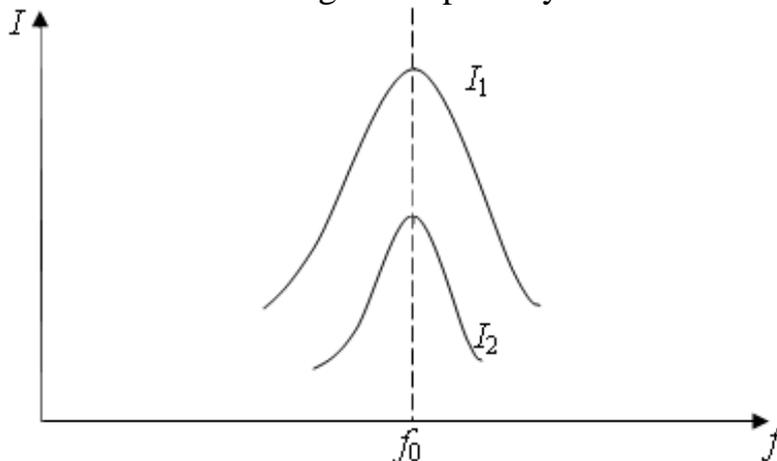
Fig. 1.22. Dependence of currents in the primary and secondary circuits on the setting of the primary circuit
