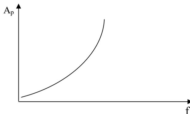
*Fig. 2.38. Attenuation characteristics of the RC-filter of low frequencies*
