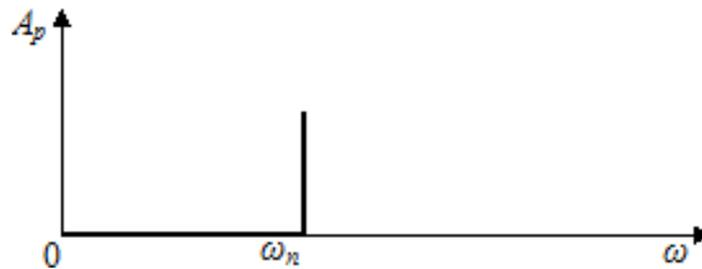
Fig. 2.7. Characteristics of the working attenuation of an ideal low-pass filter
