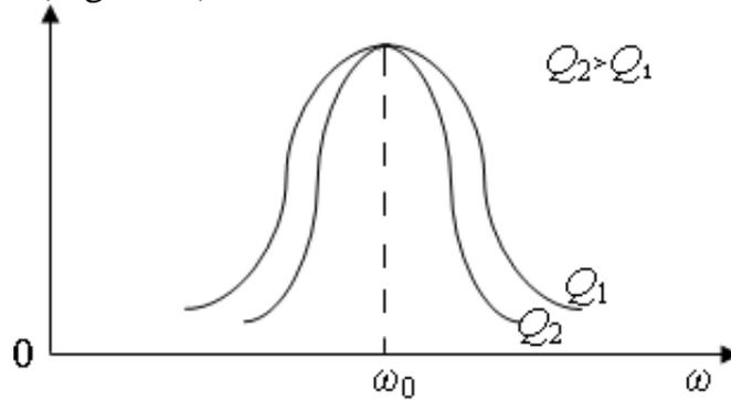
Fig. 1.14. Resonance characteristics of oscillating circuits
