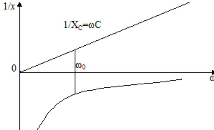
Fig. 1.4. Dependence of reactive conductivity of inductance and capacitance on frequency
