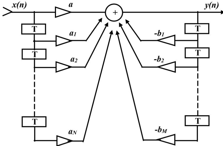
Fig. 2.64. Direct structural scheme of the IIR filter
