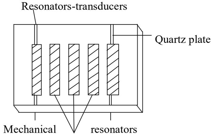
Fig. 2.35. Monolithic quartz filter
