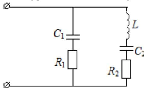
Fig. 1.26. oscillating circuit of the III type
