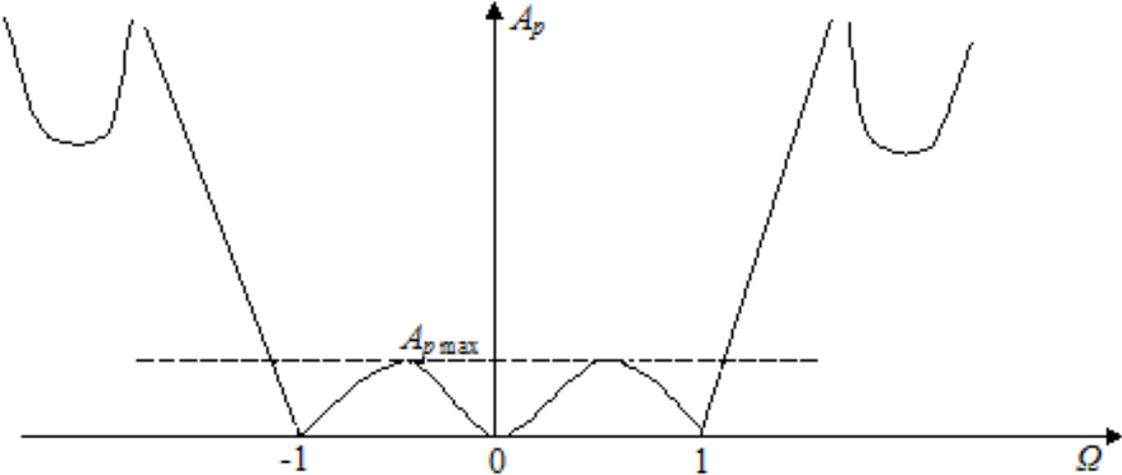
Fig. 2.19. The attenuation characteristic of the low-pass filter is symmetrical with respect to the ordinate axis
