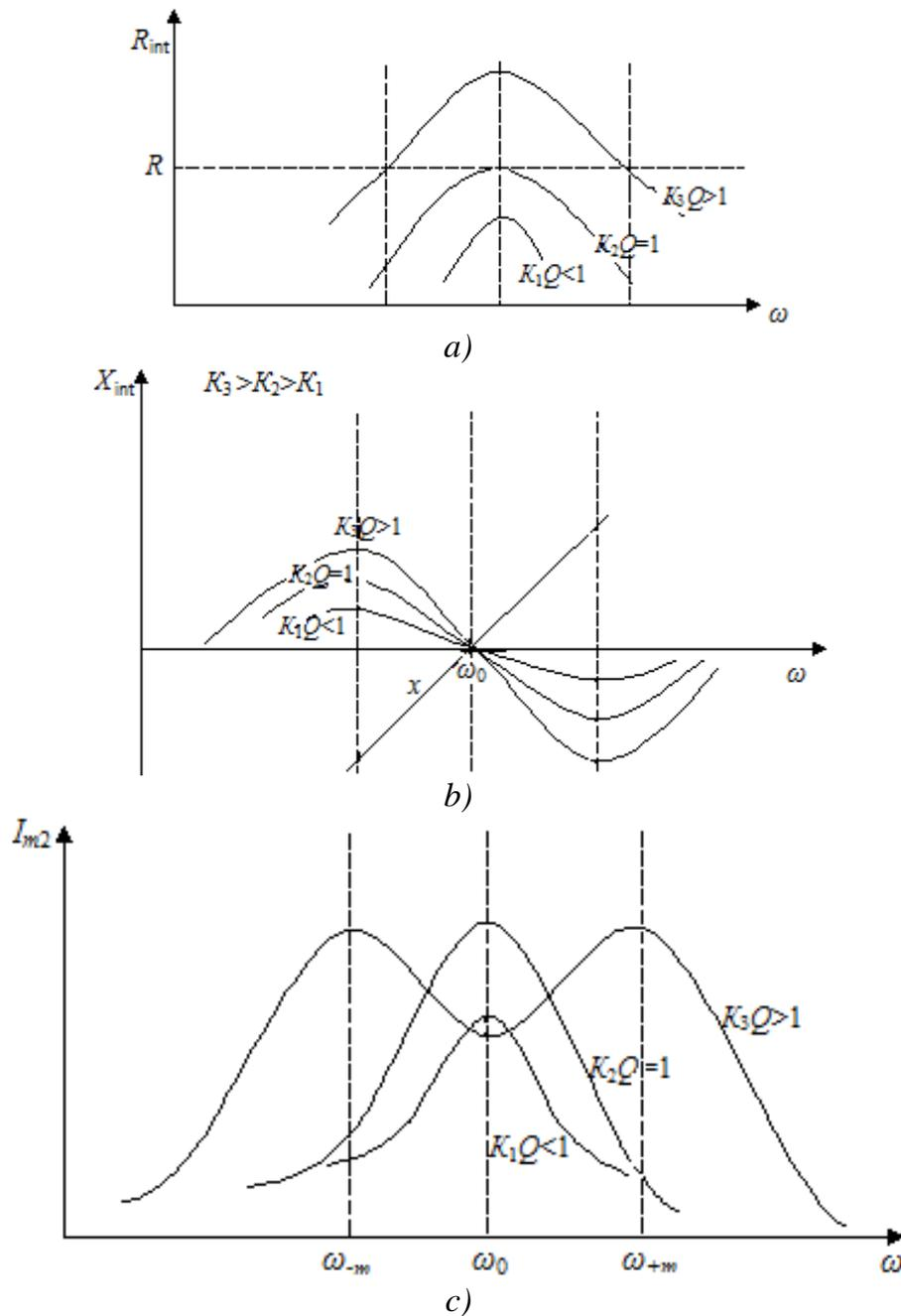
Fig. 1.20. AFC of connected oscillatory circuits for different degrees of connection
