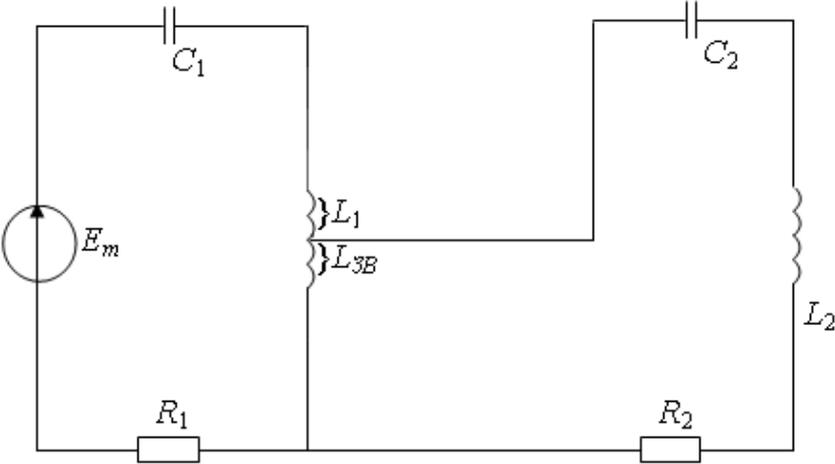
*Fig. 1.19. Connected oscillating circuits with an autotransformer connection*
