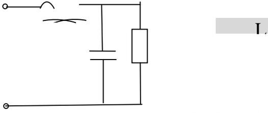
Fig. 2.43. L-shaped link of the LPF
