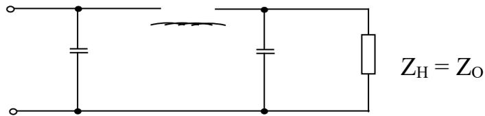
Fig. 2.27. Load of the filter on the characteristic resistance
