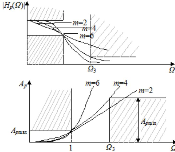
Fig. 2.9. AFC and operational attenuation of Butterworth filters
