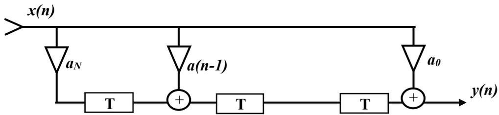
Fig. 2.63. The equivalent form of the structural scheme of the FIR filter
