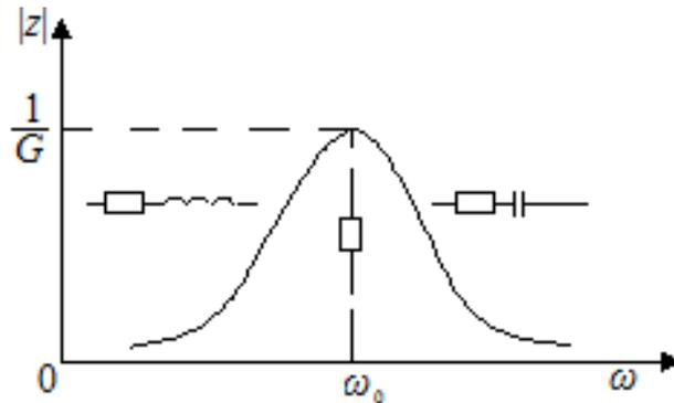
Fig. 1.8. Dependence of the resistance of the parallel oscillating circuit on the frequency
