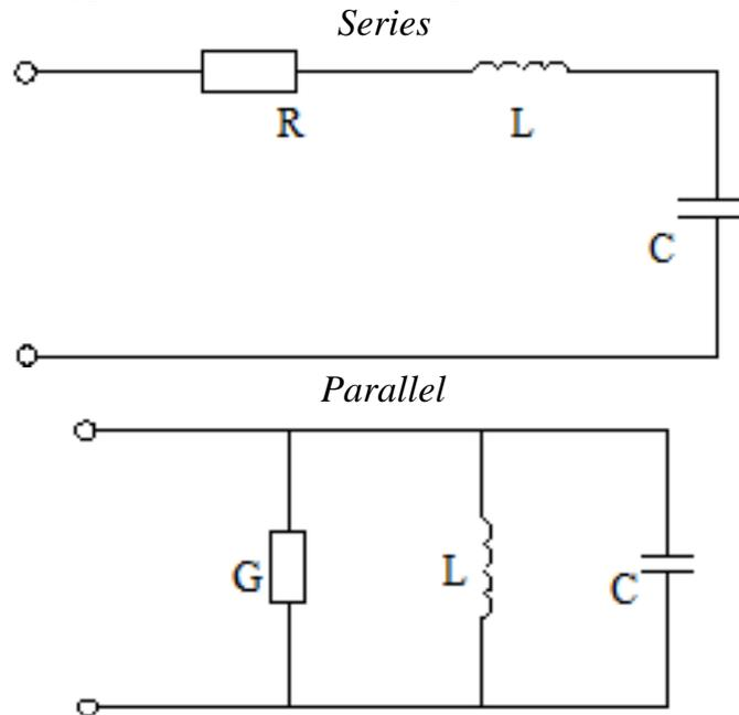
Fig. 1.1. Series and parallel oscillating circuits
