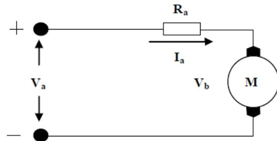
Fig. 2. Equivalent circuit for PMDC
