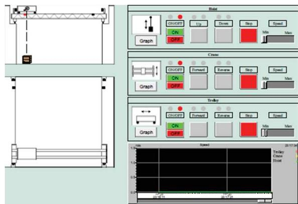
Fig. 3. HMI of simulation and contactor logic simulation
