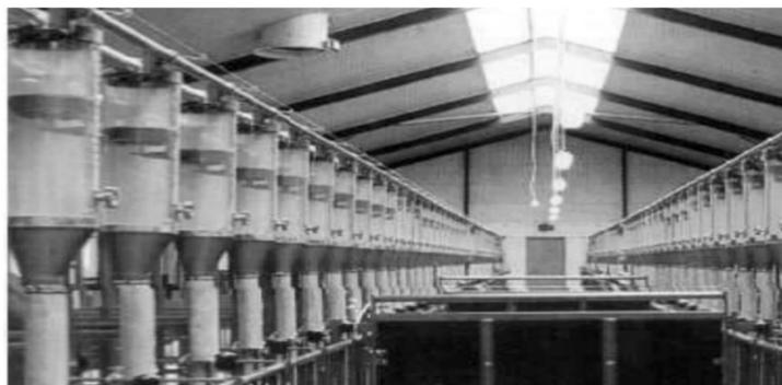
Figure 1.5 – Premises with vertical filling dispensers
