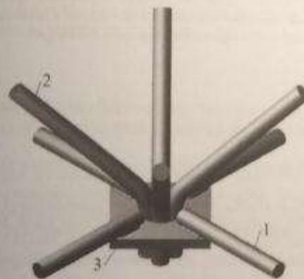
Fig. 1. Welded node of space grid structure: 1 – bottom chord; 2 – slanted rods; 3 – steel plate (by G. M. Gasii)
