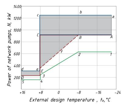
Figure 10. Power of network pumps in the heating network vs. external temperature (the corresponding options are described in the text)
