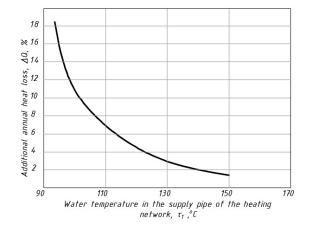
Figure 2. Additional heat losses, corresponding to the corner of the temperature curve, vs. network water temperature
