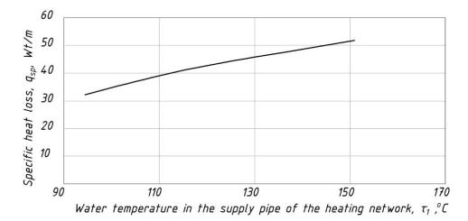
Figure 3. Specific heat losses by heating network pipes vs. network water temperature
