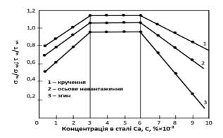
Figure 2 – Fatigue resistance ratio based on N = 107cycles in salt water (5% NaCl) in the torsion test (1), axial load (2) and bending (3)
