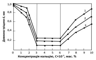
Figure 5 – The effect of calcium concentration on the crack length in the axial section of the sample: 1 - when tested for bending deformation; 2 - axial load; 3 - torsional deformation
