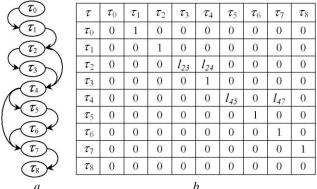
**Fig. 3:** Group technology model: *a* is the structure and parameters graph, *b* is the adjacency matrix of elements;  $\tau_0 \dots \tau_8$  are technological operations, 0 is falsity, 1 is the truth;  $l_{23}$ ,  $l_{24}$ ,  $l_{45}$ ,  $l_{47}$  are logical expressions. With its orderly sequence
