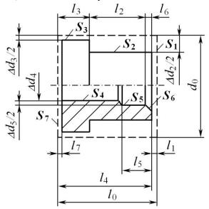
**Fig. 4:** Parametric Model of Complex Detail  $D_1: S_1 \dots S_7$  – treated surface,  $\Delta d_j$  and  $l_j$  is the change in the diameter of the surface during its treatment and the length of the cutting,  $d_0$  and  $l_0$  are the diameter and length of the initial direct circular cylinder.
