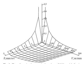
**Fig. 1:** Three-dimensional geometric dependency F(S, V) model: S – innings, V – cutting speed.
