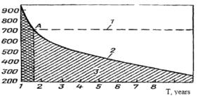
**Fig. 3:** The change in the allowable flow rate, which prevents the formation of hydrates, in the process of field development: 1 is the allowable flow rates line; 2 is the project flow rate; 3 is the hydrates zone
