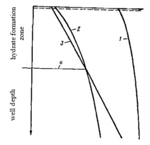
**Fig. 2:** Determination of the zone of possible formation of hydrates, where 1 is a well pressure; 2 is equilibrium temperature of hydrate formation; 3 is temperature in the well; 4 is the depth of the neutral layer
