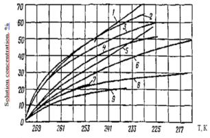
Fig. 4: The dependence of the freezing point of water on the concentration of the solution. Inhibitors: 1 - glycerin; 2 - TEG; 3 - DEG, 4 - EG; 5 -  $C_2H_5OH$ ; 7 - NaCI; 8 - CaC12; 9 - MgCl<sub>2</sub>
