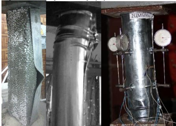
Fig. 3: Experimental samples of three-component steel-reinforced concrete constructions during testing: reinforced LSTC profile of open section, steel-reinforcement concrete constructions CSCS40, CSCS150
