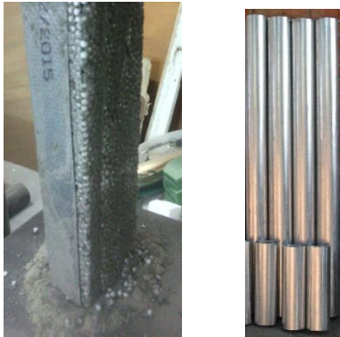
Fig. 2: Experimental samples of the three-component steel reinforced concrete structures: reinforced LSTC profile of open section, steel-reinforced concrete structures CSCS40, CSCS150
