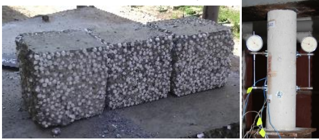
Fig. 1: Experimental samples of polystyrene concrete
