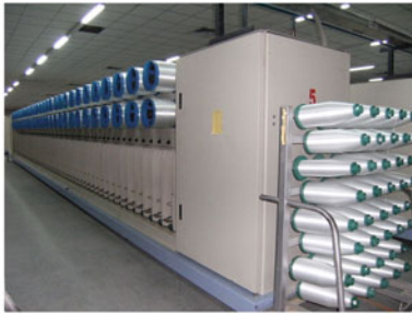
rewinding of fiber glass filament
