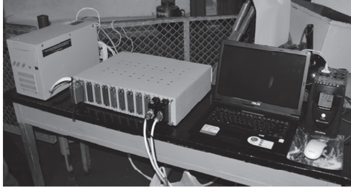
Pic. 2. Multichannel measuring tensometric system for static tests Layout of instrumentation for the study of the normal cross section (pic. 3).
