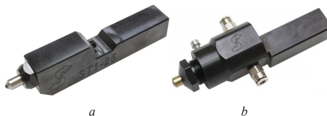
Fig. 3. Equipment of various designs for diamond smoothing of the ST series: a – fixed preload is provided; b – cooling is provided, in addition
