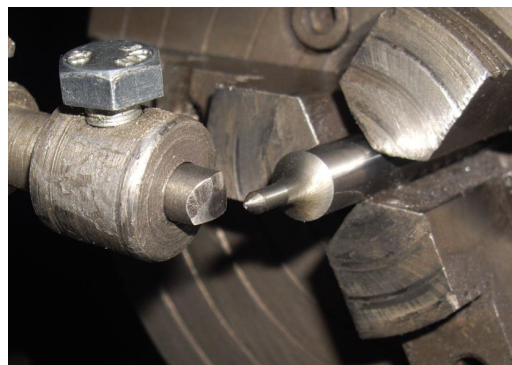
Fig. 6. Pre-installation of the mandrel for diamond knurling
