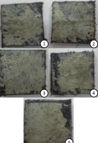
**Fig. 2:** Initial appearens of specimens of the form with a layer of hardened cement mixture (after the production process)
