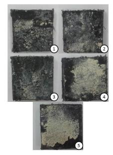
**Fig. 3:** The appearens of the form samples with a layer of hardened cement mixture (after the production process) after the first treatment with the appropriate mixtures
