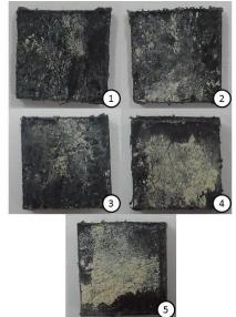
**Fig.5:** The appearens of the form samples with a layer of hardened cement mixture (after the production process) after the third treatment with the appropriate mixtures
