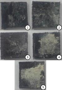
**Fig. 6:** The appearens of the form samples with a layer of hardened cement mixture (after the production process) after the fourth treatment with the appropriate mixtures
