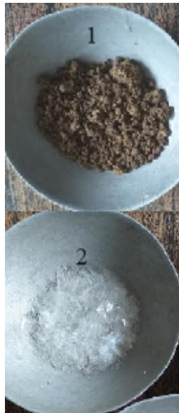
Figure 1. General view of the components of the mixture: 1 - loess loam; 2 - crushed plastic waste (2 mm).
