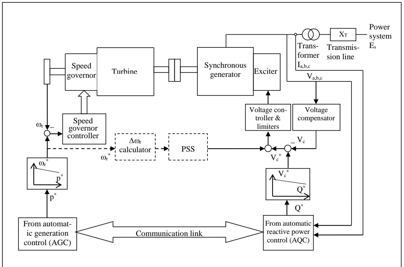
Fig. 1: General synchronous generator control system
