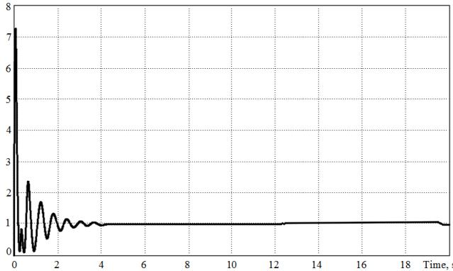
Fig. 13: Generator current (pu) with Time (s)
