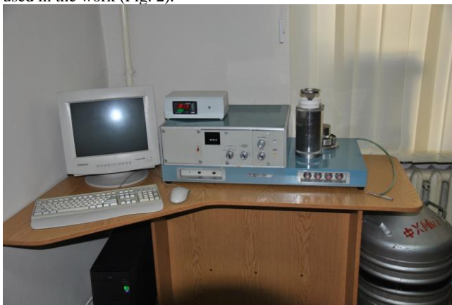
Fig. 2: The differential scanning microcalorimeter DSM-2M
