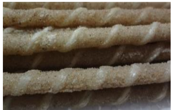
Fig. 2: General view of fiber-glass reinforcement
