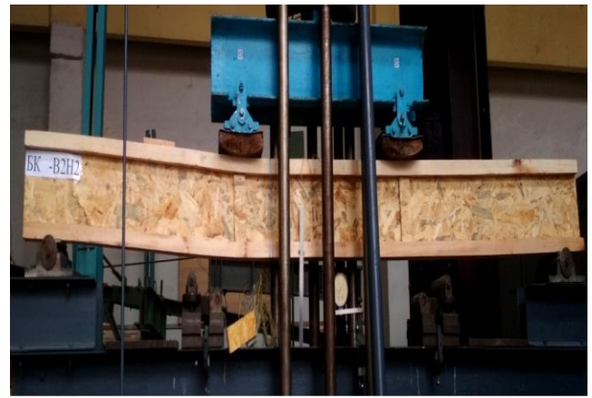
Fig. 10: Beam “БК-Н2В2” after destruction
