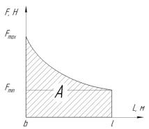
Fig. 5: The dependency diagram of the force acting on the piston from the path that it travelled, giving up energy:
