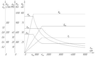
**Fig.7:** Initial characteristics of the hydrostatic transmission of the tractive unit with an adjustable pump and, regulable hydraulic oil motor:
