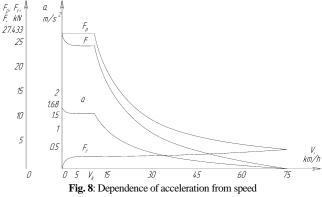
One hydraulic accumulator is fully charged and discharged at 7.33 turns of the tractive unit wheel (with the capacity of a hydraulic accumulator - 16 liters). That is, the gas volume in the battery is proportional to the path that the car has traveled since the start of the movement with the drive from the battery or since the beginning of regenerative braking.
