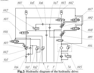
T – tank; HA1, HA2 – hydraulic accumulator APX-16/320; HM1,HM2 – A6V hydraulic oil motor; Va1, Va2 – safety valve 510.32; Va3 – back-pressure valve 61100; Va4-Va7 – back-pressure valve 61400; P1- pump A7V; P2 – pump NCH 6T-1; HV1-HV8 – hydraulic valve; TA – heat-transfer apparatus KM6-CK-1; F – filter 1132-25.
