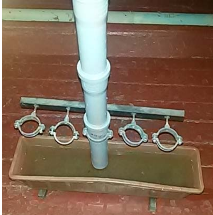
Fig. 4.2 – Chute, filled with water for possible capillary ascension research for road embankment
