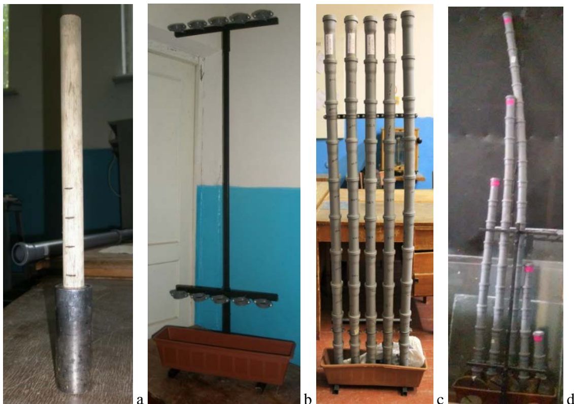
Fig. 3.2 – Stages of compacted subgrade loam moisture conditions laboratory studies: a – hand tamper for soil compaction; b – vertical frame for pipe placement with compacted; c, d – pipes, filled with compacted soil with marks upper about initial soil skeleton density \rho_d and its required moisture w
