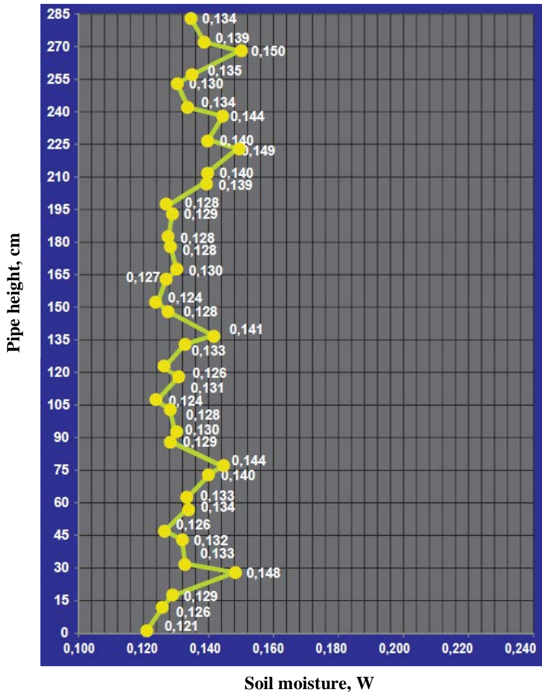
Fig. 3.5 – Moisture plot changes of compacted light silt loam heightwise the pipe of 2,85 m at soil skeleton density 1,55 g/cm 3
