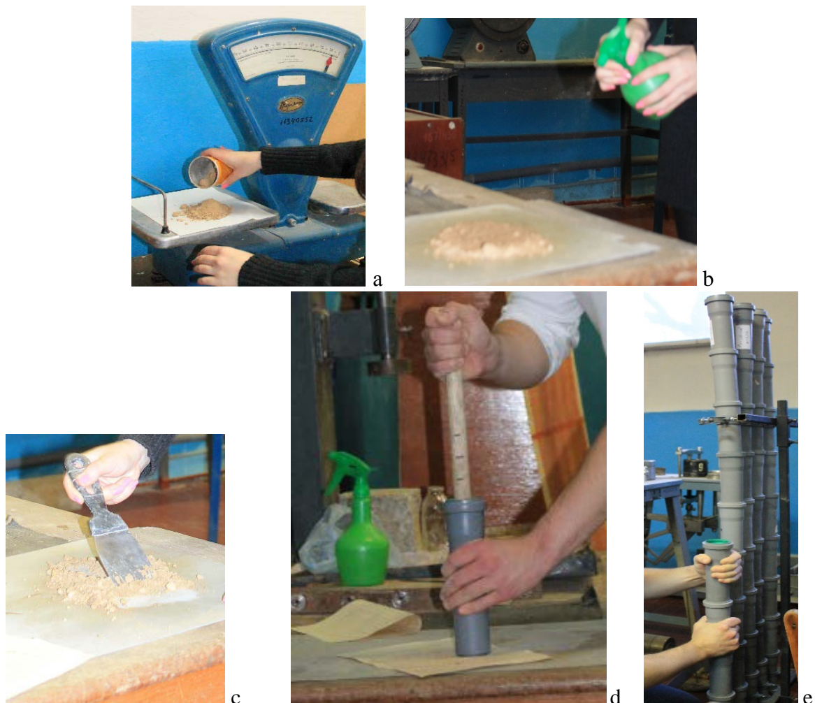
Fig. 3.1 – Stages of compacted road embankment loam moisture conditions laboratory studies: a – weighting an appropriate research soil mass portion; b – additional moistening of clay soil portion to a given value w ; c – research soil mixing for it's uniform moistening; d – multilayer (3 cm) compaction of each loam portion; e – erected to a common pipe links height
