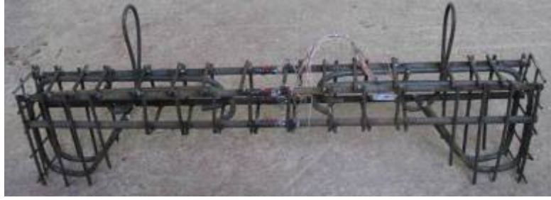
Figure 4 – Spatial reinforcing cage for reinforced concrete columns
