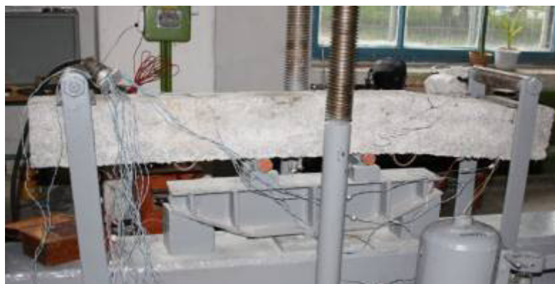
Figure 9 – Investigation of beam 1B – FC – 1 on flexure
