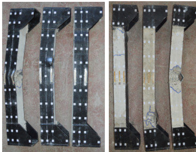
Figure 5 – The destruction nature of experimental steel-concrete samples with sheet reinforcement of the series SB-PD-10-1..3 and SB-PN-10-1..3
