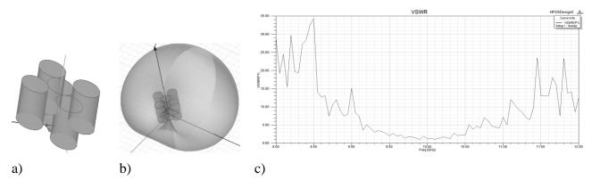
Fig. 2. The first version of quasifractal DRA: a) – power circuit; b) – BP; c) – frequency dependence of a SWR
