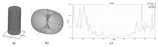
Fig. 1. Basic element of the DRA on the basis of a cylinder: a) – power circuit;b) – BP; c) – frequency dependence of a SWR
