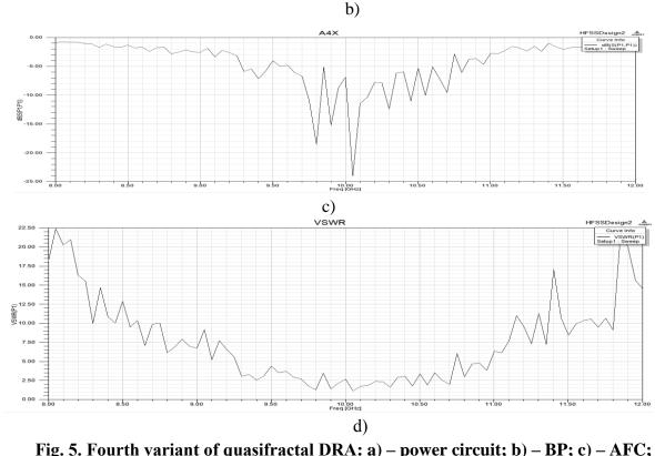
Fig. 5. Fourth variant of quasifractal DRA: a) – power circuit; b) – BP; c) – AFC; d) – SWR
