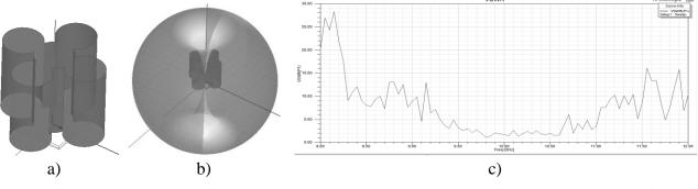
Fig. 3. The second version of quasifractal DRA: a) – power circuit; b) – BP; c) – frequency dependence of a SWR
