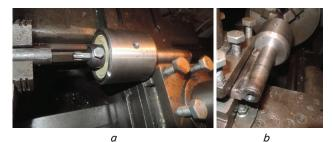
Fig. 3. Rotational head from rotating center: a - view of rotational head; b - method of fixing in the tool carrier
