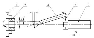
Fig. 2. Kinematic schematic of the work of rotational head for broaching the profile openings: 1 - chuck of lathe;
