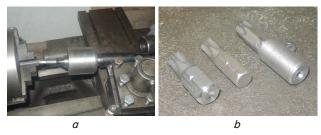
Fig. 4. Fabrication of profile openings with tool selfcentering: a – making profile openings; b – bit-centering technique
