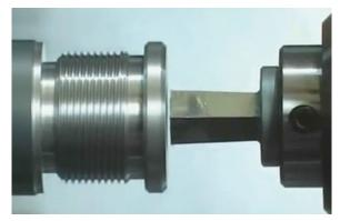
Fig. 1. Broaching of profile opening on the lathe
