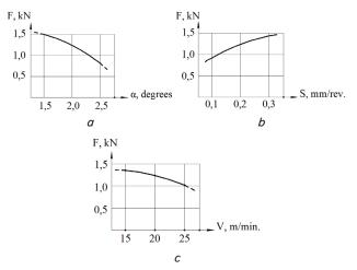
Fig. 6. Dependence of pressing force F, kN: α - on the tool entrance angle α, degrees (S=0.2 mm/rev; V=20 m/min); b - on the tool supply S, mm/rev (α=2 degrees; V=20 m/ min); c - on the process rate V, m/min (α=2 degrees; S=0.2 m/min)
