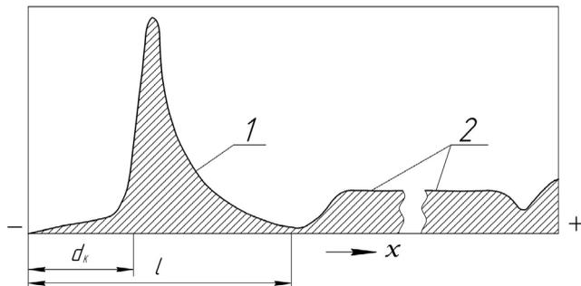
Fig. 1. The intensity distribution of discharge plasma radiation, that glow, with flat parallel gap:
