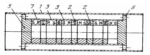
Picture 2 – Schematic diagram of a magnetic anti-paraffin unit (MAU-1) with mutually perpendicular directions of magnetization of the magnet ring:
