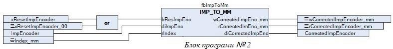
Figure 3.14 – Process control program block, number two
