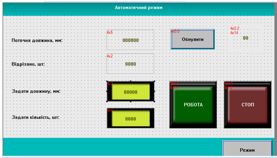
Figure 3.7 – Programmed automatic mode of operation of the machine
