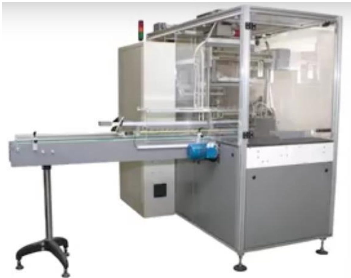
Figure 1.5 – Packing machine for boxes with tea in cellophane
