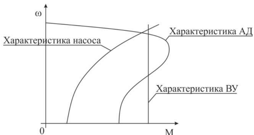
Figure 1.2 - Mechanical characteristics of AD, pump and VU
