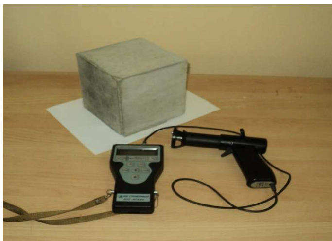
Figure 1. Determination of compressive strength using the device IPS-MG- 4.03
