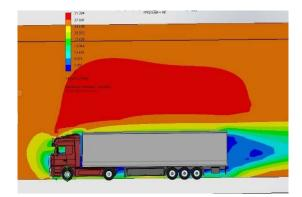
Figure 3 – Diagram of air speed distribution around the road train at a speed of 100 km/h
