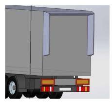
Figure 6 – Model of the Mercedes-Benz Actros car with a rear wing-skirt
