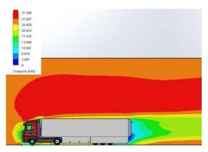
Figure 11 – Diagram of wind speed distribution around a road train at a speed of 100 km/h with a fairing of the lower part of the trailer and a Henning-Marxen bag tail and an rear wing
