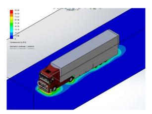
Figure 13 – Diagram of air vorticity distribution around a road train at a speed of 100 km/h with the fairing of the lower part of the trailer and the tail with a Henning Marxen bag and an rear wing
