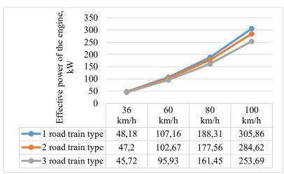
Figure 14 – Dependence of engine power for different types of road trains makings
