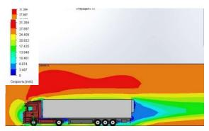
Figure 9 – Diagram of air speed distribution around the road train at a speed of 100 km/h with a wing-skirt located behind
