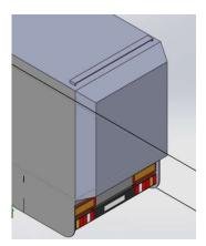
Figure 8 – Mercedes-Benz Actros car model with trailer underbody fairing and Henning-Marxen tail bag and rear wing
