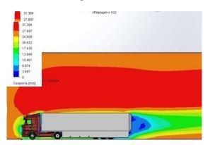
Figure 10 – Diagram of the air velocity distribution around the road train at a speed of 100 km/h with the fairing of the lower part of the trailer and the tail of the Henning-Marxen bag
