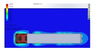
Figure 12 – Diagram of air vorticity distribution around a road train at a speed of 100 km/h with a fairing of the lower part of the trailer and a Henning-Marxen bag tail
