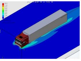
Figure 4 – Diagram of air vorticity distribution around the road train at a speed of 100 km/h
