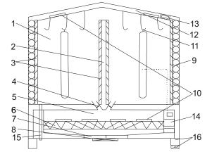
Fig. 1. Scheme of the design of the universal apparatus for heat treatment of combined meat and vegetable products:
