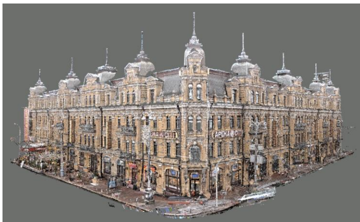
Fig. 2. The result of 3D scanning with a laser scanner
