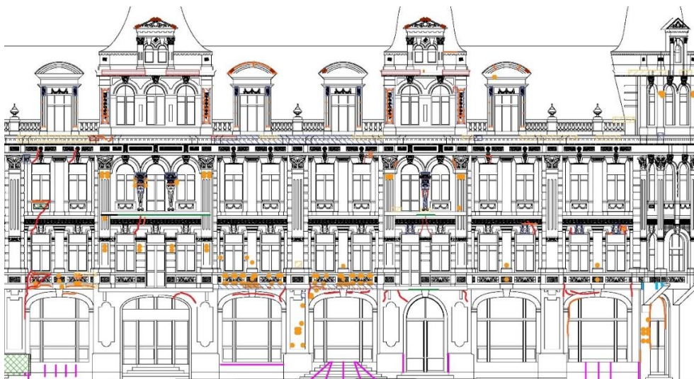
Fig. 5. A fragment of the facade of the building with applied defects and damage.
