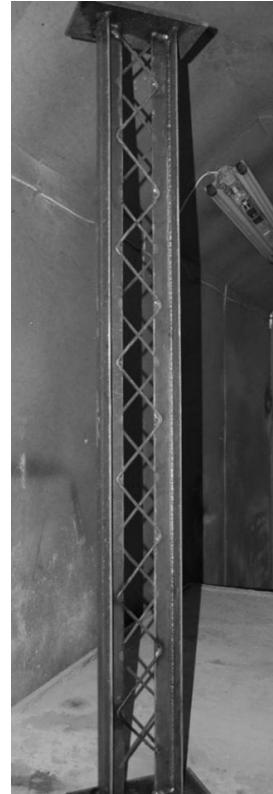
FIGURE 1. Design of the experimental samples (a) and General view of the samples before concreting (b).
