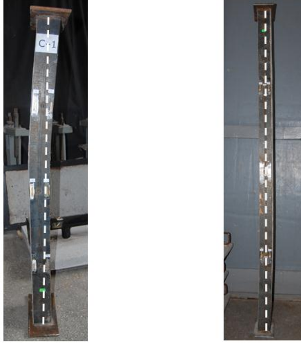
FIGURE 4. General view for sample C1 after testing.
