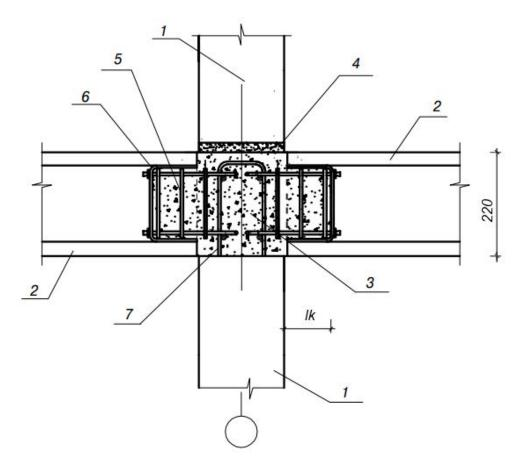
Fig. 1 Combined joint of multi-hollow slabs with wall panels: 1 – wall panel; 2 – floor slab; 3 – cast-in-place concrete; 4 – mortar; 5 – key reinforcement frame; 6 – plastic plug; 7 – reinforcement outlets from wall panels;  $l_k$  – the length of floor suspension (calculated value)
