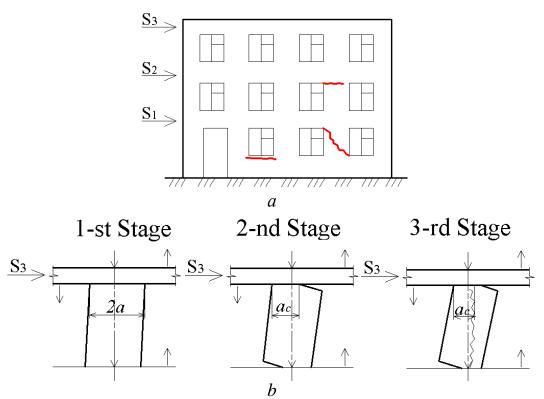
Figure 1 - The work of the walls of the bearing walls under the action of a horizontal seismic force:
