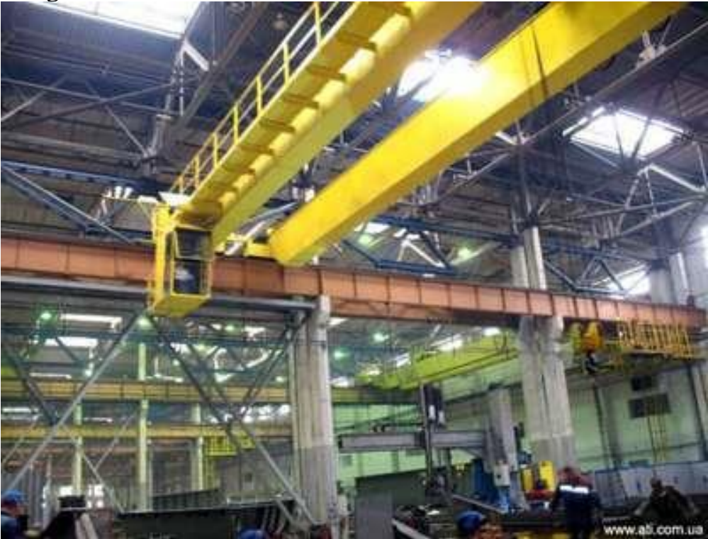
Fig. 13.2. Overhead travelling double-girder crane
