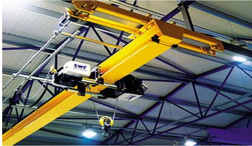
Fig. 13.7 Underslung crane (runway beam for hoist block)
