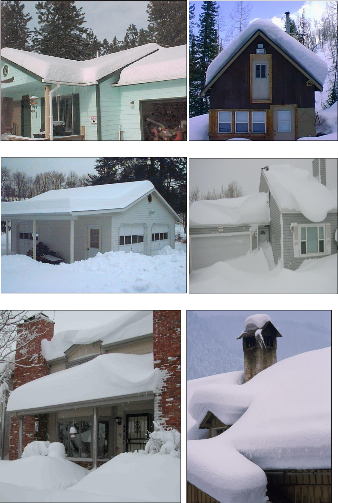
Fig. 10.8. Snow load on sloping roofs
