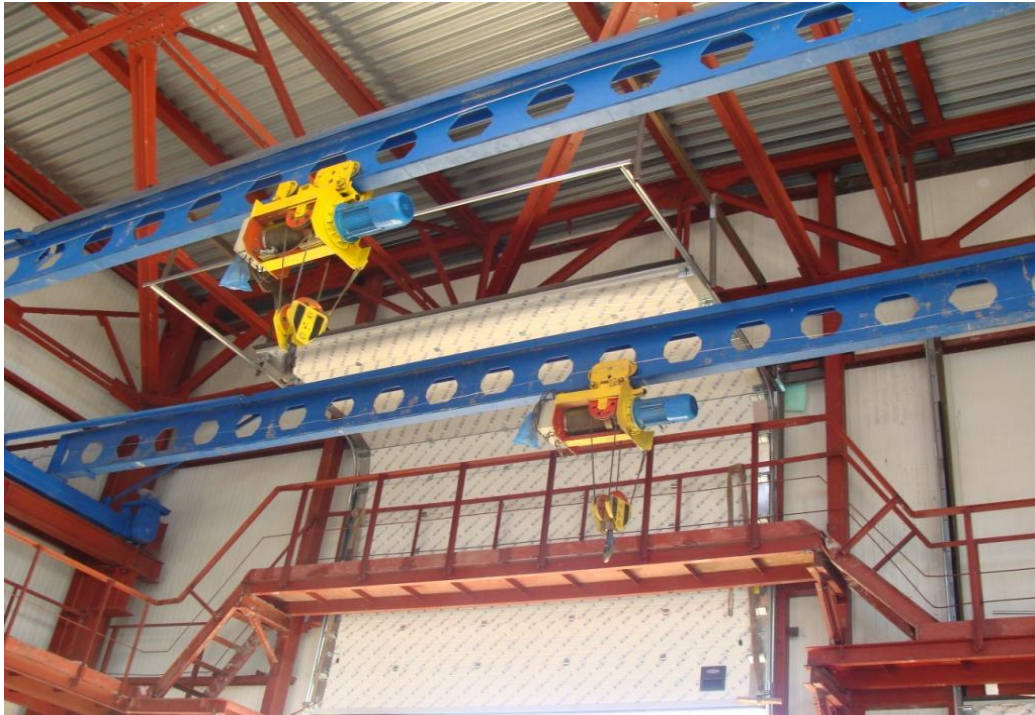
Fig. 13.1 Single-girder crane (with perforated beam)
